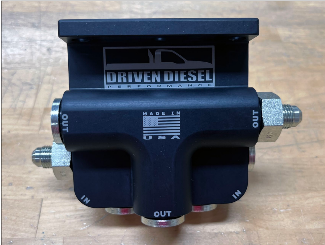
Figure 1 – Filter Head with Fittings and Plugs – Inside the Frame Flow Direction
