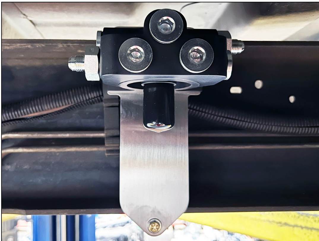
Figure 2 – Filter Bracket Mounted Inside Frame Rail
